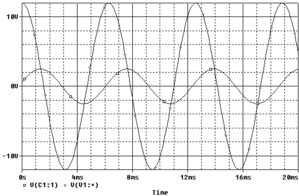
Some points on the output plot:  $v_o(0.00132) = 2.5$  V (max  $v_o$ ) and  $v_o(0.00446) = -2.5$  V (min  $v_o$ );  $v_o(0) = 0.6048$  V.
